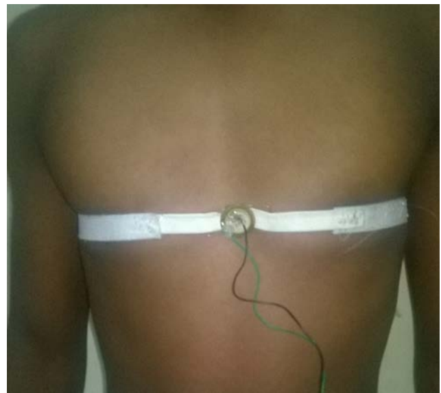
Fig 4 .Respiratory Belt placed on the chest
